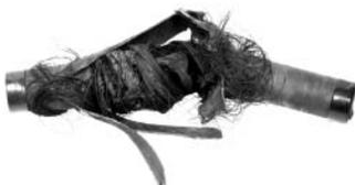
**Cause:** The hose is too short to accommodate the change in length occurring while it is pressured.
