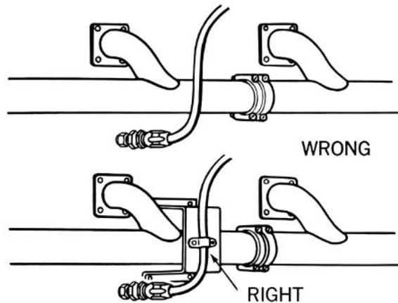
When hose lines pass near an exhaust manifold or other heat source, they should be insulated by a heat resistant boot, firesleeve or a metal baffle. In any application, brackets and clamps keep hoses in place and reduce abrasion.
