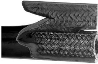
**Cause:** This would indicate a high frequency pressure impulse condition. SAE impulse test requirements for a double wire braid reinforcement are 200,000 cycles at 133% of recommended working pressure. The SAE impulse test requirements for a four spiral wrapped reinforcement (100R12) are 500,000 cycles at 133% maximum operating and at +250°F (121°C). If the extrapolated impulses in a system amount to over a million in a relatively short time a spiral reinforced hose would be the better choice.
