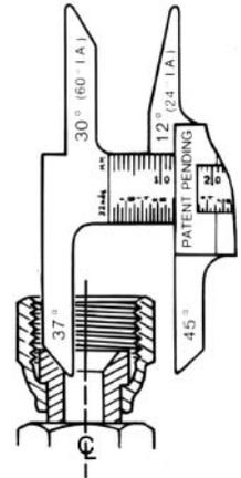
Male flare type connectors are usually measured by placing the gauge on the sealing surface. If the centerlines of the connection and gauge are parallel, the correct angle has been determined.
