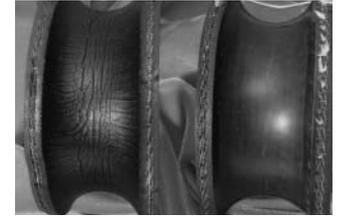
**1. Symptom:** The hose tube is very hard and has cracked.
