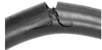
**2. Symptom:** The hose is cracked both externally and internally but the elastomeric materials are soft and flexible at room temperature.
