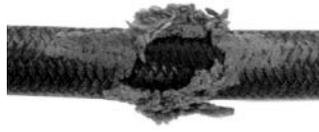
**Cause:** The primary function of the cover is to protect the reinforcement. Elements that may destroy or remove the hose covers are:
