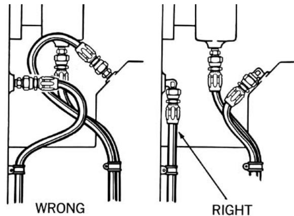
When 90° adapters were used, this assembly became neater-looking and easier to
