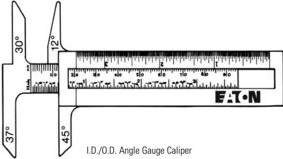
I.D./O.D. Angle Gauge Caliper
